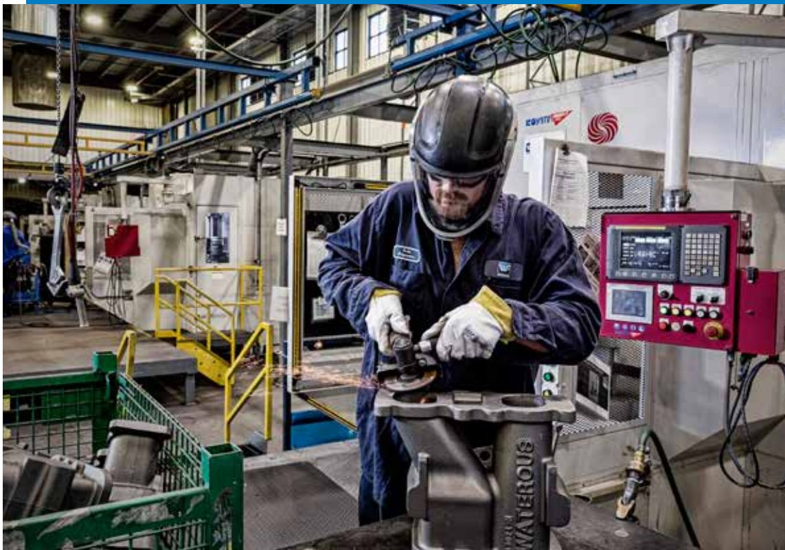
Millroom operator Kevin Klotzbuecher inspects a municipal casting before loading it into the barinder machine.
