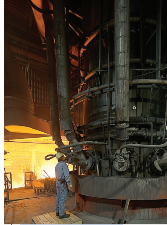
A Waupaca Foundry melt operator checks the cupola tuyeres at its Tell City, Ind., foundry.
