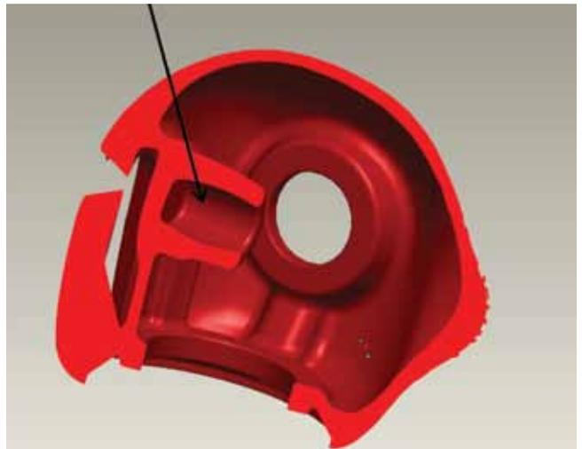
**Because simulation software predicted a large section of porosity in the solid section at the top of the hydrant, a hole was added to aid in solidification, as indicated by the arrow at right.**
